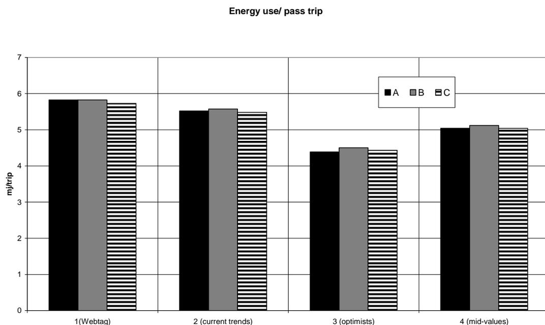
**Figure 7: Energy use by test and technology scenario**
